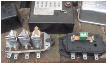
Spot the dummy? Original Control Box on left. A "Dummy" box is supplied with the Dynalite
